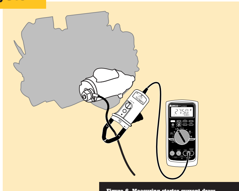
Figure 6. Measuring starter current draw
