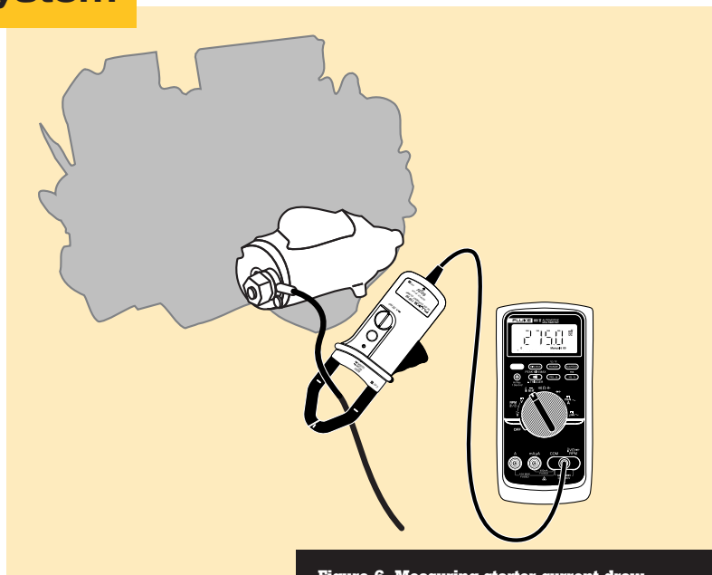
Figure 6. Measuring starter current draw
