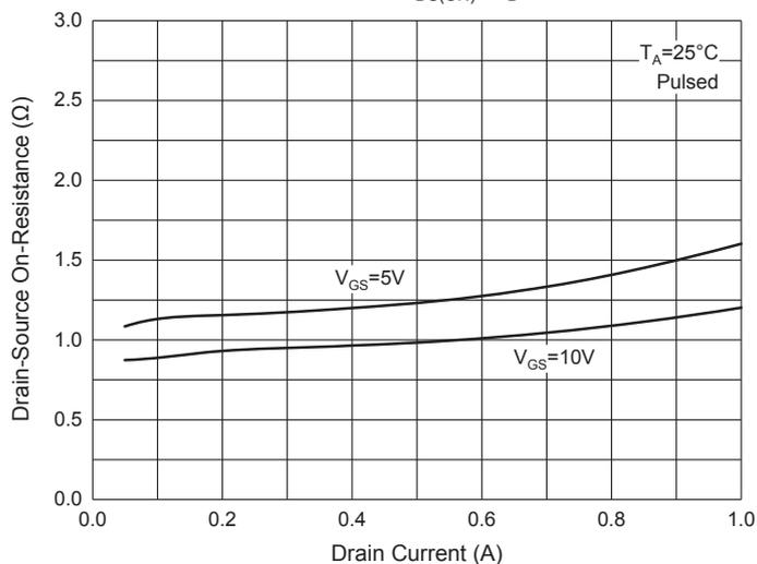
Fig. 3 -  $R_{DS(ON)} - V_{GS}$
