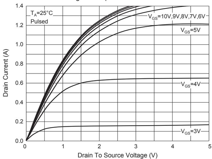
Fig. 2 - Transfer Characteristics
