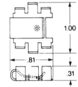
**VERTICALLY MOUNTED HEAT SINKS WITH BOARD-MOUNTED TABS**
