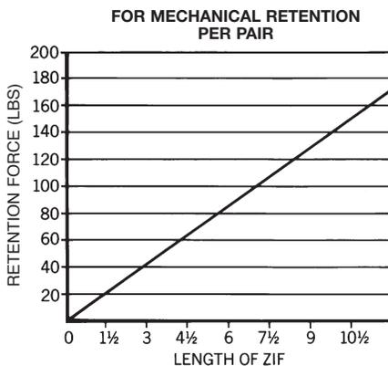
Clamping pressure is not only essential to heat transfer, but also a critical requirement for retention of PCBs under severe shock and vibration. ZIF retainers have been subjected to the most extreme test conditions specified in MIL-STD-810C.
