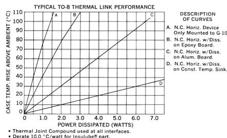
**HEAT SINKS FOR METAL AND PLASTIC CASE, CASE-MOUNTED SEMICONDUCTORS**
