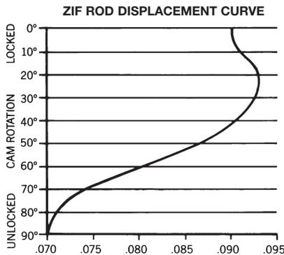
The ZIF cam detent design gives added assurance that a PCB will remain securely locked in position even under extreme vibration and shock levels. Detent action occurs during the final 15 degrees of cam rotation and virtually eliminates any possibility of the cam unlocking under environmental stress.
