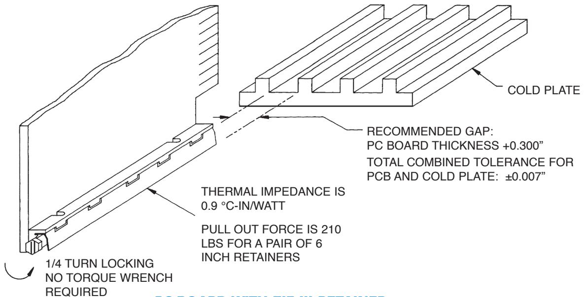
**PC BOARD WITH ZIF III RETAINER**
