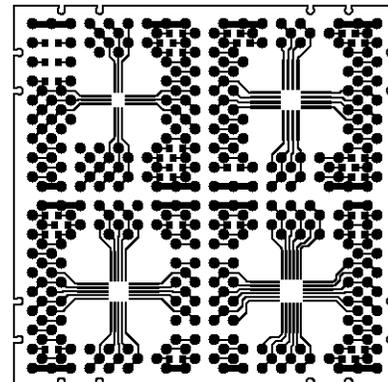
Supports .5mm Pitch 12, 20 and 24 Lead QFNs & 16 Lead .65mm QFN. A hole in the center of each gives access to a ground or thermal pad on IC.
