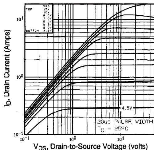
**Fig. 1 - Typical Output Characteristics,  $T_C = 25^\circ\text{C}$**
