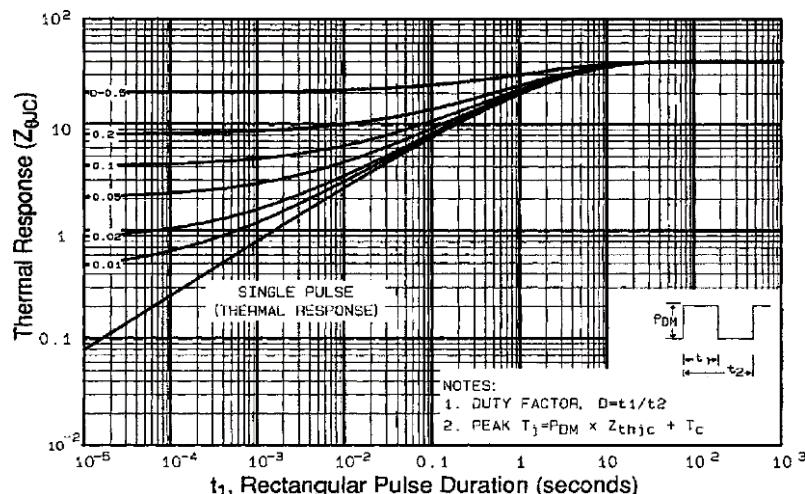
Fig. 11 - Maximum Effective Transient Thermal Impedance, Junction-to-Case
