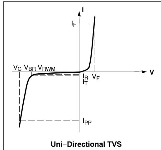
**ELECTRICAL CHARACTERISTICS** ( $T_A = 25^\circ\text{C}$  unless otherwise noted)
