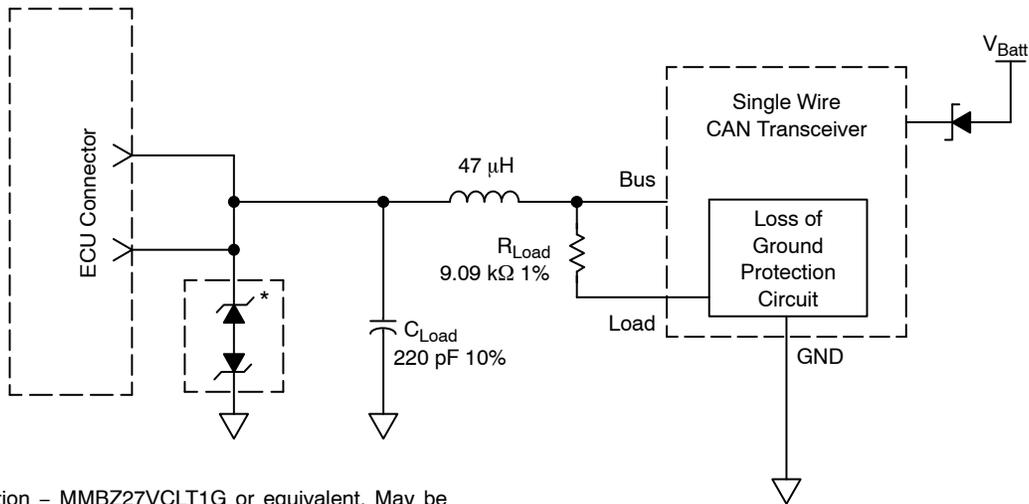
\*ESD Protection – MMBZ27VCLT1G or equivalent. May be located in each ECU ( $C_{Load}$  needs to be reduced accordingly) or at a central point near the DLC.
