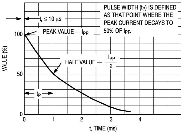
**Figure 5. Pulse Waveform**
