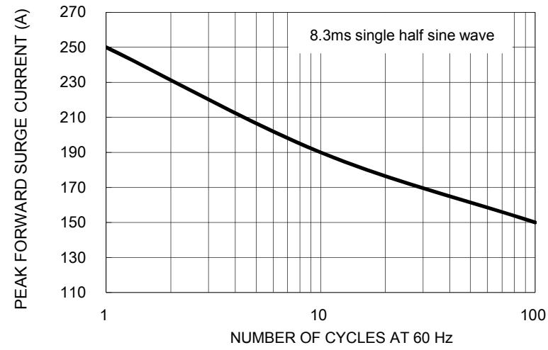
FIG. 7 MAXIMUM NON-REPETITIVE PEAK FORWARD SURGE CURRENT
