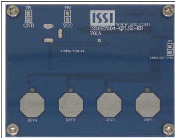
Figure 1: Photo of IS31SE5104 Evaluation Board
