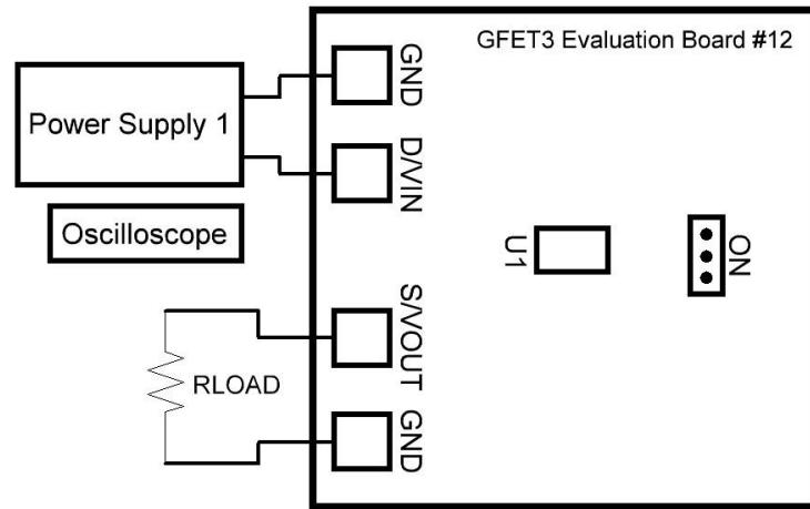
**Figure 5. Typical connections for GFET3 Evaluation**
