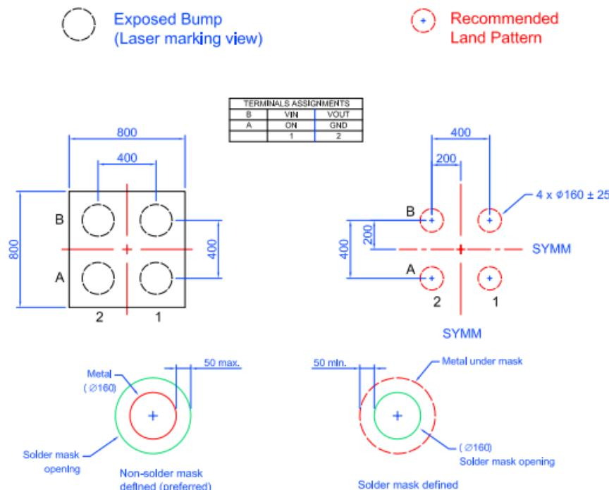
**Figure 2. SLG59M1730C Package Dimensions and Recommended Land Pattern**
