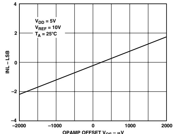
Figure 10. Linearity Error vs. External Op Amp Vos
