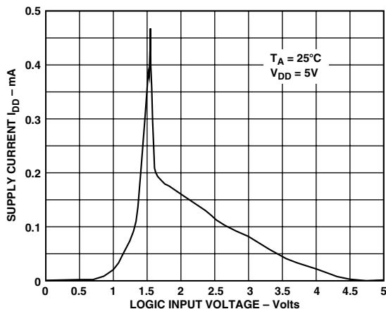
Figure 5. Supply Current vs. Logic Input Voltage
