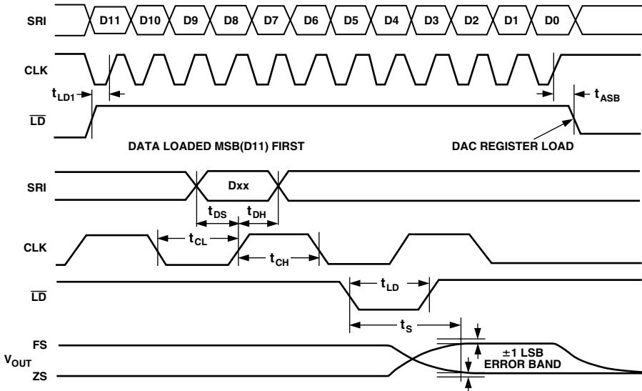
Figure 2. Timing Diagram
