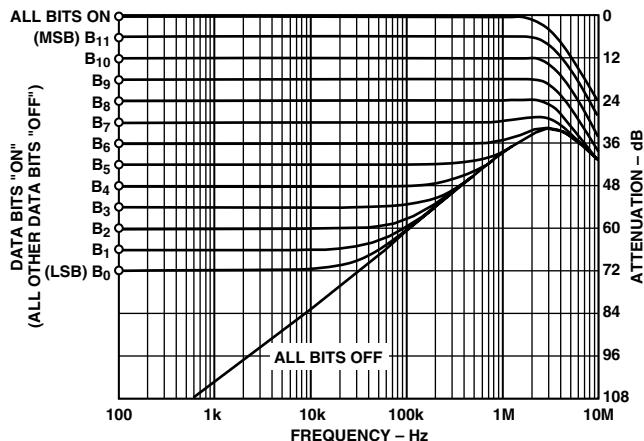
Figure 13. Reference Multiplying Bandwidth vs. Frequency and Code
