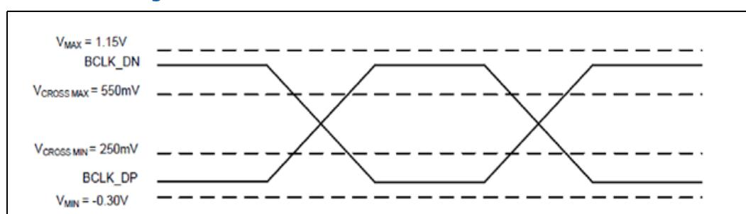
**Figure 2-8. BCLK{0/1/2} Single Ended Clock Measure Points for Delta Cross Point**
