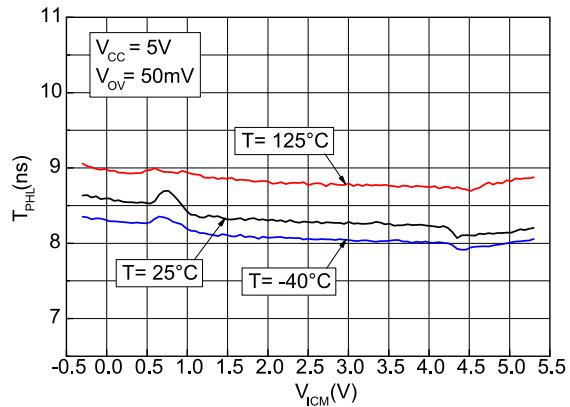
**Figure 11: Propagation delay vs. common mode voltage with positive transition**
