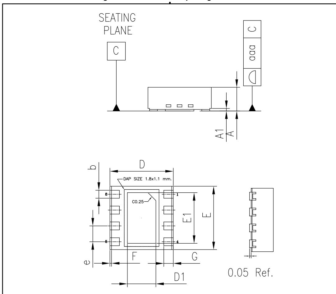
Table 8: DFN8 2x2 mm package mechanical data
