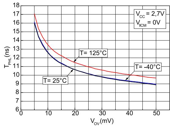
**Figure 15: Propagation delay vs. overdrive with positive transition, V<sub>CC</sub> = 2.7 V**
