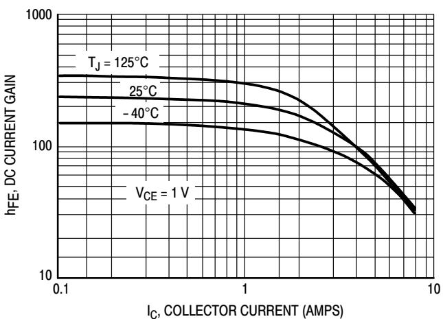
**Figure 7. MJB45H11 Current Gain versus Temperature**
