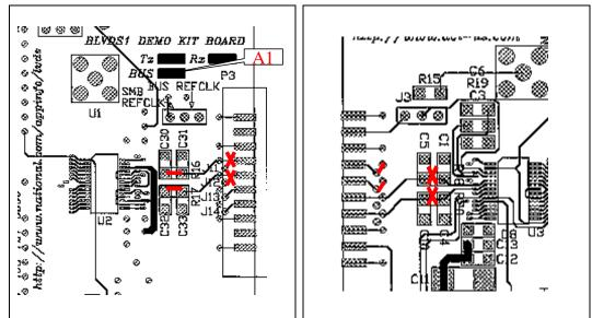
1. On the DUT card, side A, solder a jumper from the R16 pad to the inside pad of C30.
