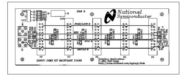
Each side of the backplane card has two differential busses, a REFCLK bus to distribute the REFCLK signal to Deserializer cards, and a SYNC/LOCK bus that connects the LOCK\* output from Deserializers to the SYNC1 input of the Serializer.
