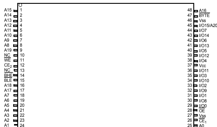
Figure 2. 48-pin TSOP I pinout (Top View) [2, 3]
