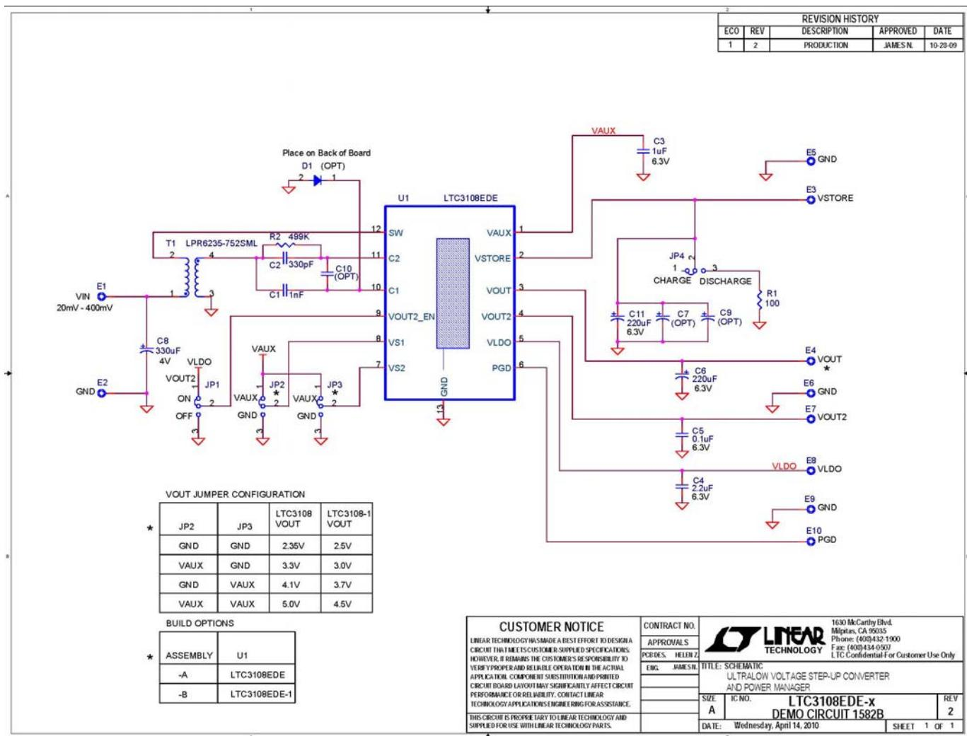
Figure 3. Circuit Schematic
