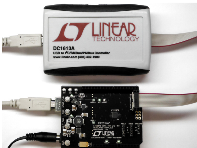
Figure 7. DC2467 with DC1613 Dongle Attached
