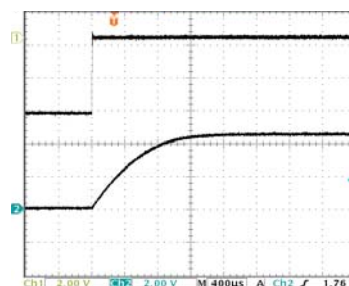
Typical Start-Up Wave Form
