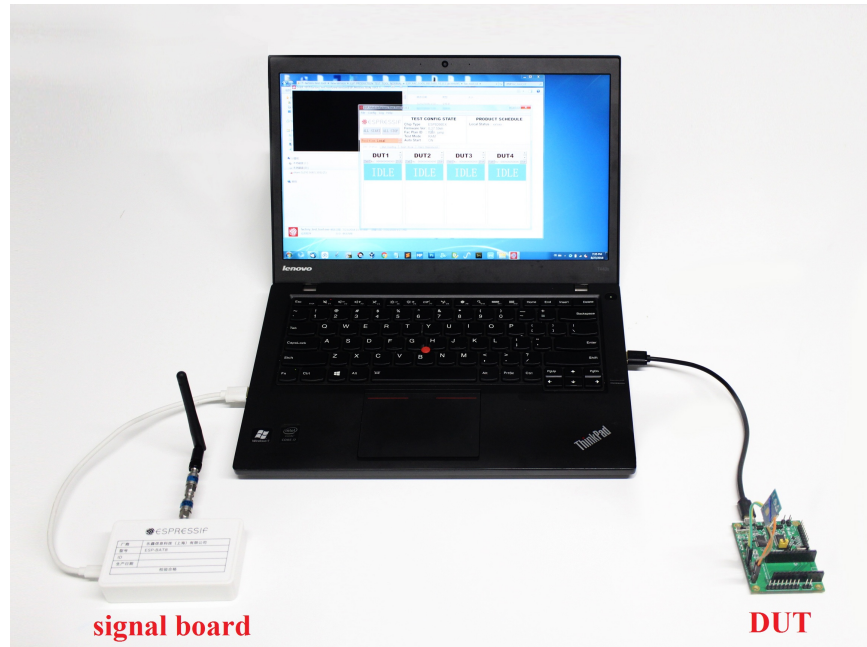
Figure 2-3. Quick Start on Testing Diagram
