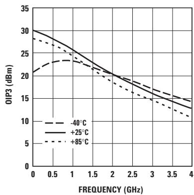
Figure 9. Output IP3 vs. Frequency and Temperature.
