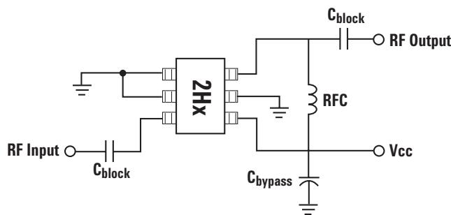
Figure 1. ABA-52563 Production Test Circuit.
