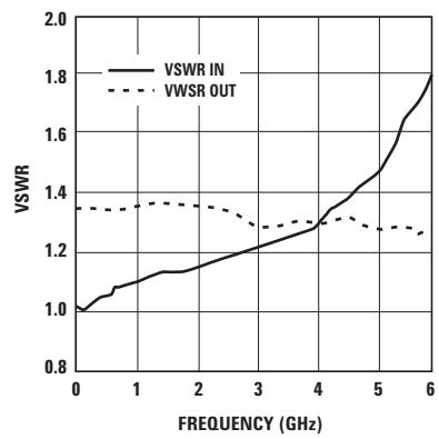
Figure 10. Input and Output VSWR vs. Frequency.
