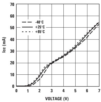
Figure 11. Supply Current vs. Voltage and Temperature.
