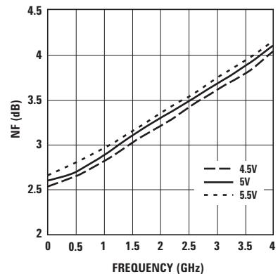
Figure 4. Noise Figure vs. Frequency and Voltage.
