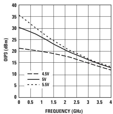
Figure 8. Output IP3 vs. Frequency and Voltage.
