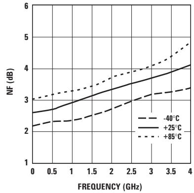
Figure 5. Noise Figure vs. Frequency and Temperature.
