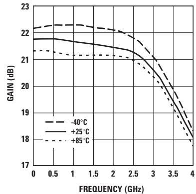
Figure 3. Gain vs. Frequency and Temperature.
