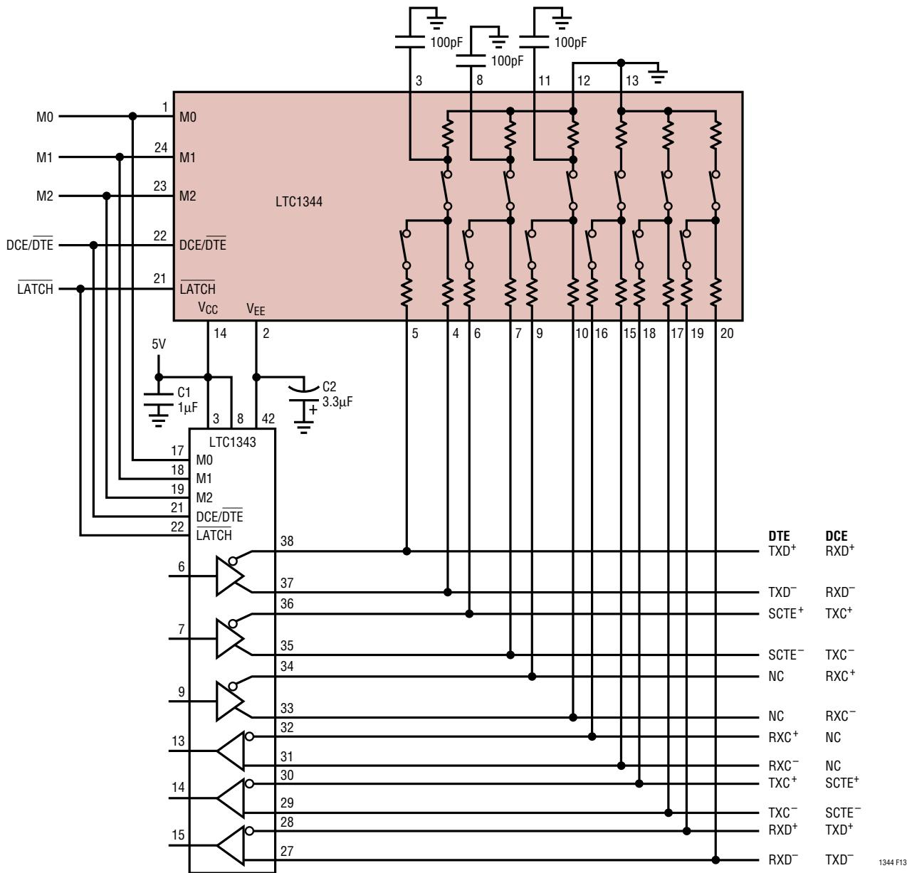
Figure 13. Typical Application Using the LTC1344
