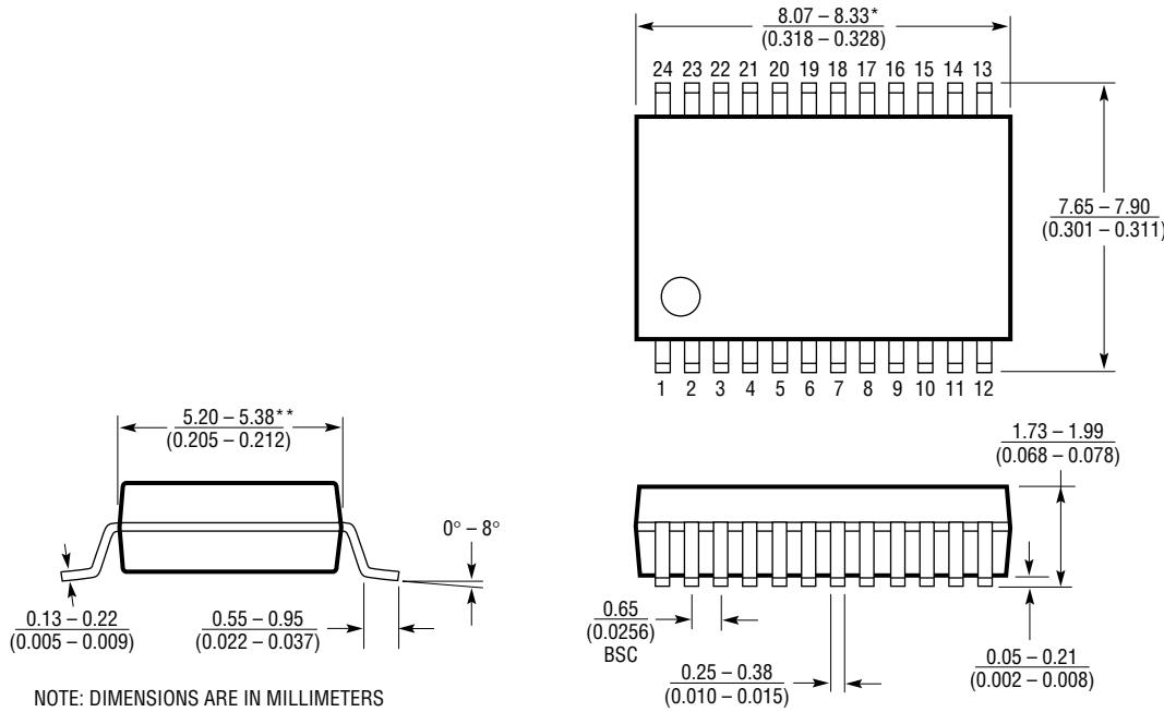
NOTE: DIMENSIONS ARE IN MILLIMETERS
