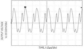
Figure 9. Typical Output Ripple and Noise (Vin = 12.0V dc, Vo = 3.3 Vdc, Io=6A).
