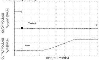
Figure 14. Typical Start-Up Using Remote On/Off (Vin = 12Vdc, Vo = 3.3Vdc, Vo = 6.0A).
