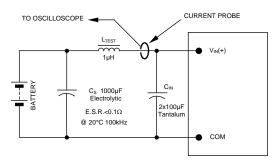
NOTE: Measure input reflected ripple current with a simulated source inductance ( $L_{\rm TST}$ ) of 1µH. Capacitor C<sub>S</sub> offsets possible battery impedance. Measure current as shown above.
