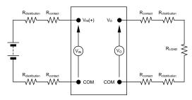
NOTE: All voltage measurements to be taken at the module terminals, as shown above. If sockets are used then Kelvin connections are required at the module terminals to avoid measurement errors due to socket contact
