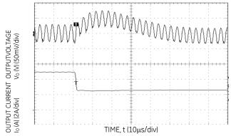
Figure 13. Transient Response to Dynamic Load Change from 100% of 50% full load (Vo = 5.0 Vdc, Cext =  $2x150~\mu F$  Polymer Capacitors).
