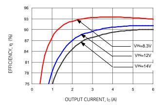
Figure 6. Converter Efficiency versus Output Current (Vout = 5.0Vdc).
