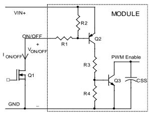
Figure 28. Circuit configuration for using positive logic On/OFF.
