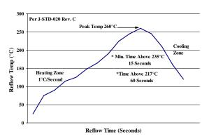
Figure 37. Recommended linear reflow profile using Sn/Aq/Cu solder.
