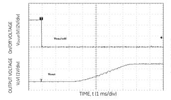
Figure 15. Typical Start-Up Using Remote On/Off with Low-ESR external capacitors (7x150uF Polymer)
