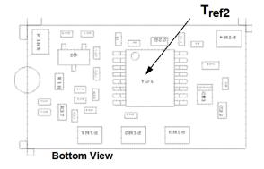
Figure 32. Tref Temperature measurement location.
