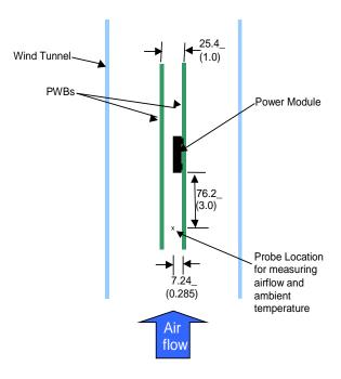
Figure 33. Thermal Test Set-up.
