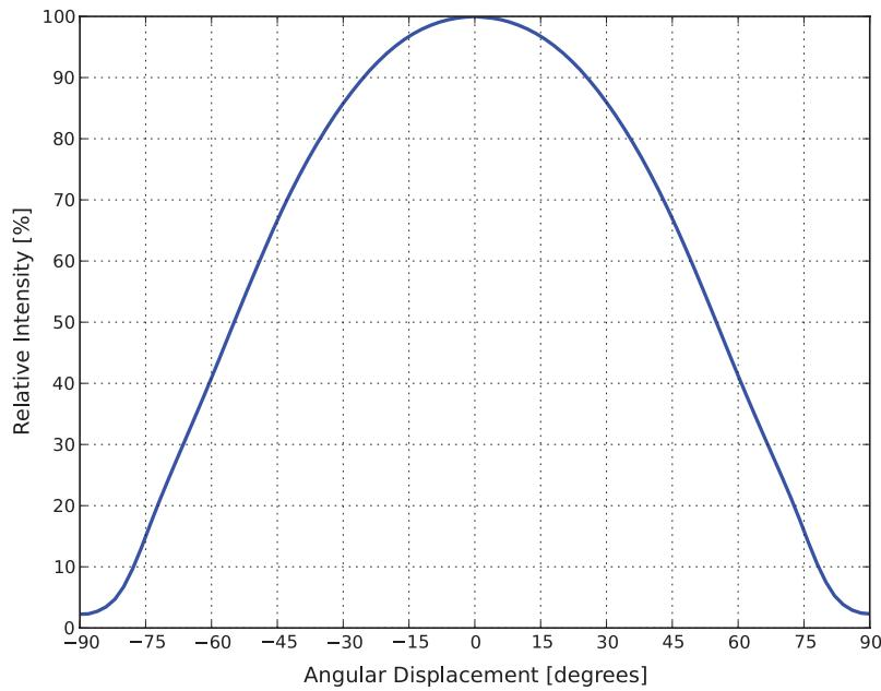
Figure 10. Typical representative spatial radiation pattern for LXAC-1xxx.
