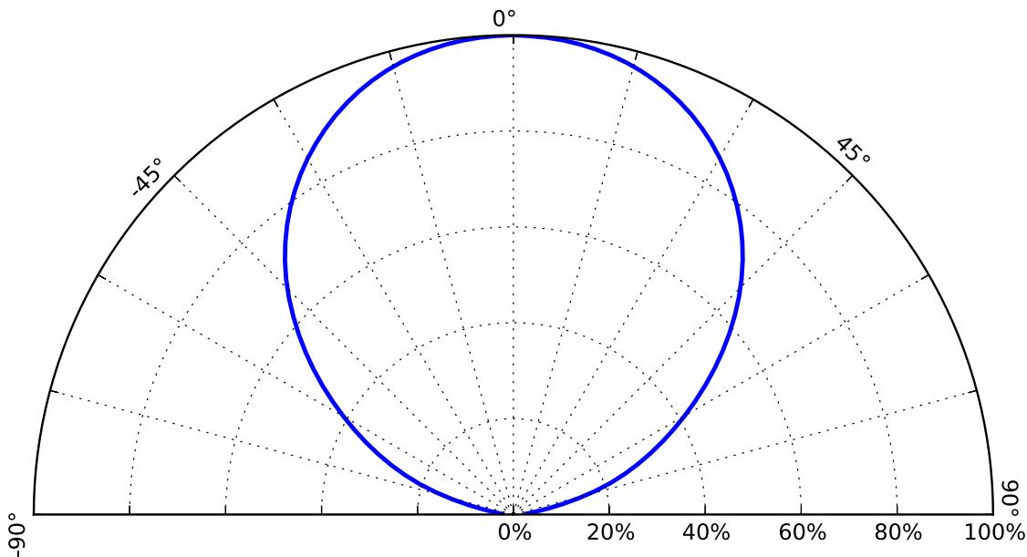
Figure 11. Typical representative polar radiation pattern for LXAC-1xxx.
