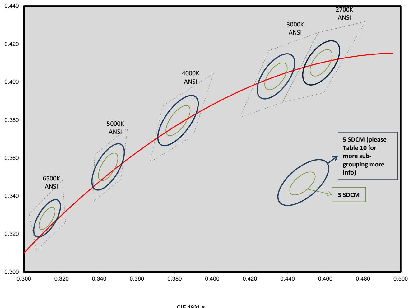
Figure 14. LUXEON H50-2 color bin structure for 2700K and 3000K.
