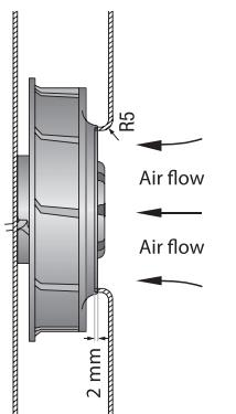
The air flow and noise level of the centrifugal fans without external housing depend on their individual installation conditions. The stated air flow and noise level were recorded under the following measurement parameters:
