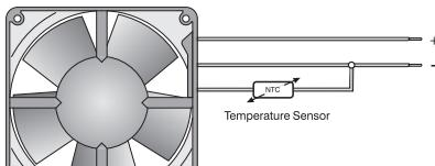
The temperature sensor for controlling the motor speed is not included in delivery.
