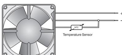
The temperature sensor for controlling the motor speed is not included in delivery.
