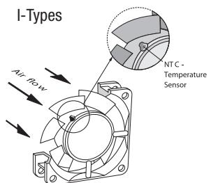
Temperature sensor (NTC-resistor) for controlling the motor speed is positioned directly in the air flow.
