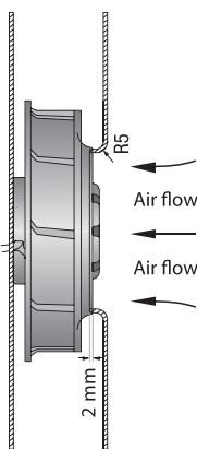
The air flow and noise level of fans without external housing depend on the installation conditions. The stated air flow and noise levels have been measured under the following conditions:
