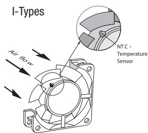
Temperature sensor (NTC-resistor) for controlling the motor speed is positioned directly in the air flow.
