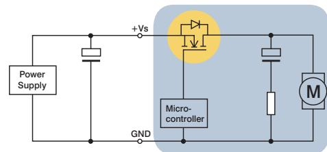
Recommended measure: Additional external capacitor (thus must be installed as close to the fan as possible < 30 cm).
