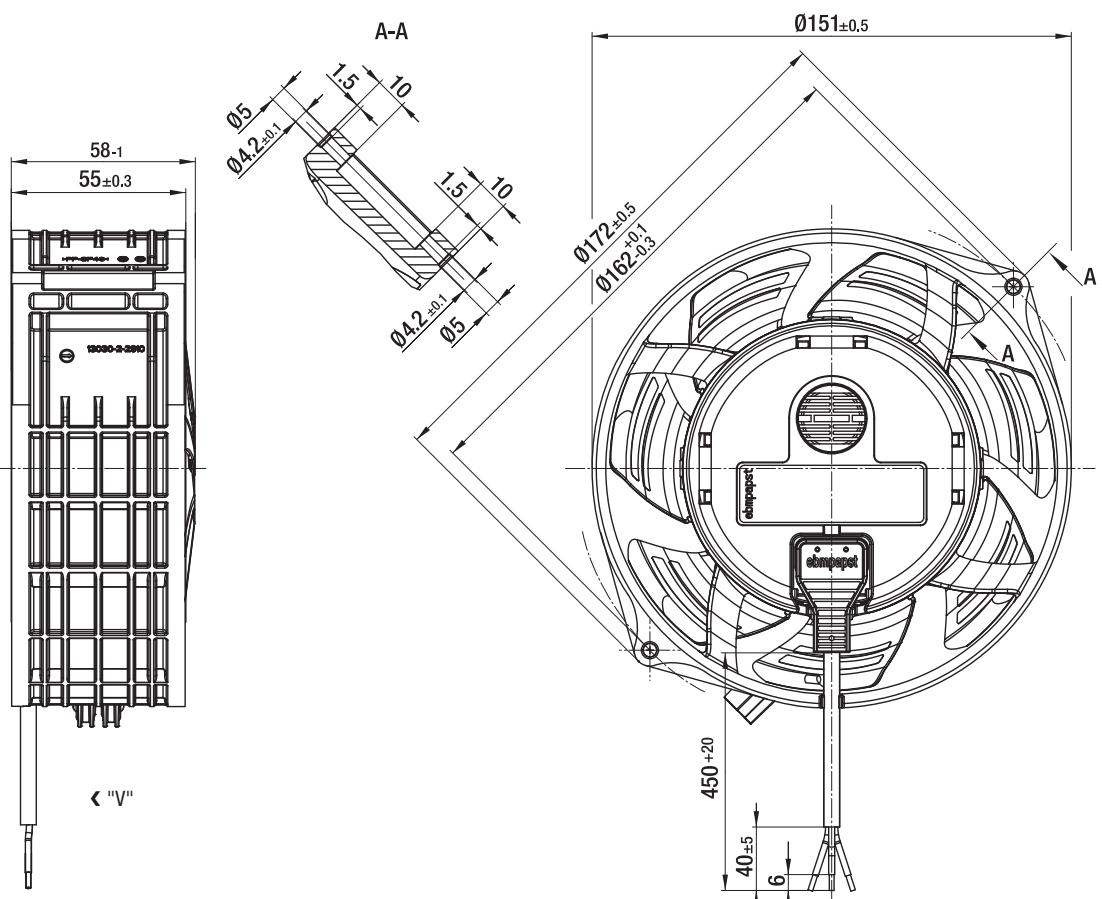
Connection lead (total length 450 mm) is fitted ex works and can be detached.
