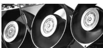
Fans in an endurance test cabinet at ebm-papst St. Georgen.
