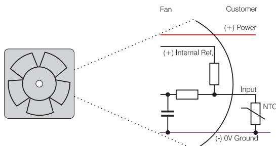
**Internal temperature sensor Type I**
