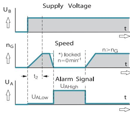
$t_2$  = Alarm signal suppression during start-up
