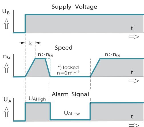
$t_2$  = Alarm signal suppression during start-up.
