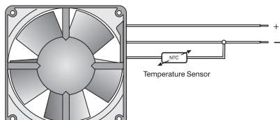
The temperature sensor for controlling the motor speed is not included in delivery.
