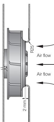
The air flow and noise level of the centrifugal fans without external housing depend on their individual installation conditions. The stated air flow and noise level were recorded under the following measurement parameters:
