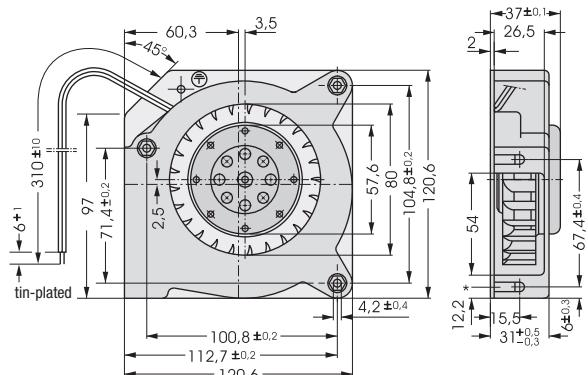
\*Speed nut M4 or 8-32UNC, Screw-in depth max, 12,5 min 9,0
