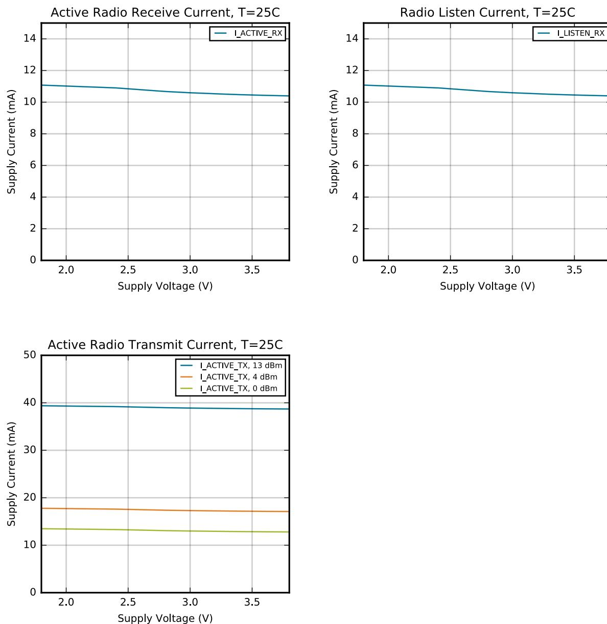
**Figure 4.1. Supply Current vs. Supply Voltage**
