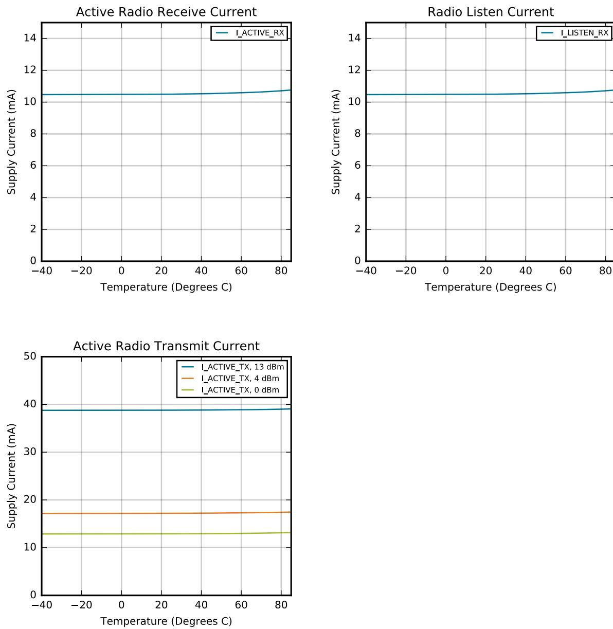
Figure 4.2. Supply Current vs. Temperature
