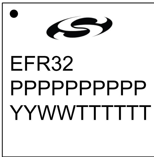
Figure 7.3. QFN32 Package Marking
