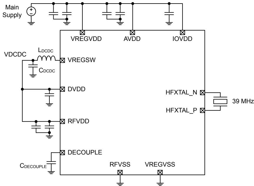
**Figure 3.1. Power Supply Connections**
