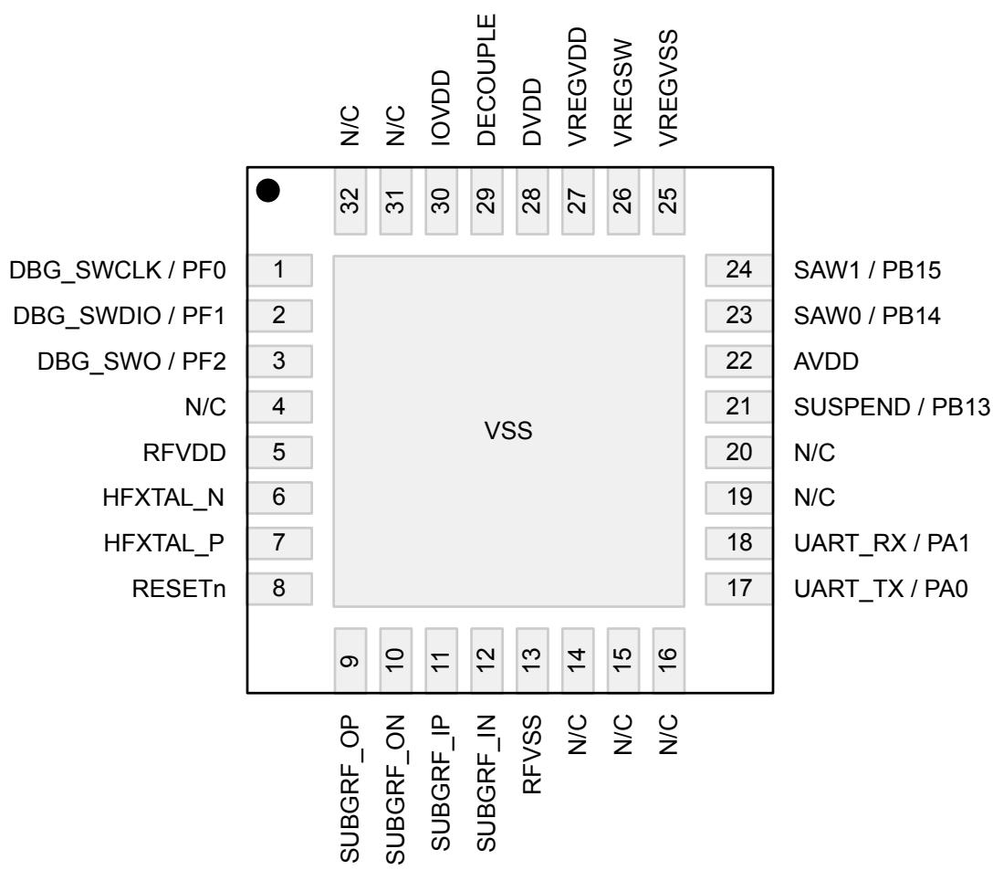
**Figure 6.1. EFR32ZG14 Device Pinout**
