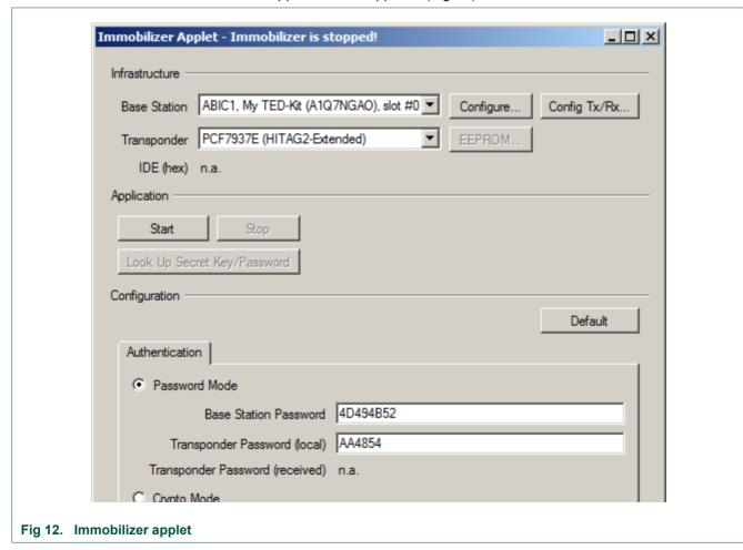
The window contains three different parts: In the upper part, the Infrastructure frame which shows the currently configured infrastructure for the applet. In the window shown
