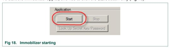
Now, the applet continuously tries to authenticate with HITAG2-Extended transponder in the antenna's field. If no transponder is in range, the Immobilizer window looks like Fig 19.
