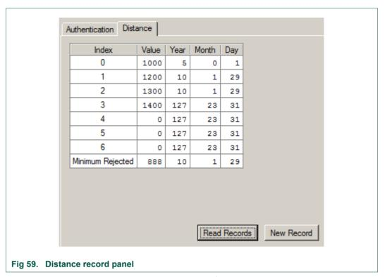
The table contains the 7 current records and the 8<sup>th</sup> record which is used as internal log. Initially, no records are read. In order to get the current values, click Read Records. To create a new distance record, click New Record and fill the data in the upcoming dialog (Fig 60).
