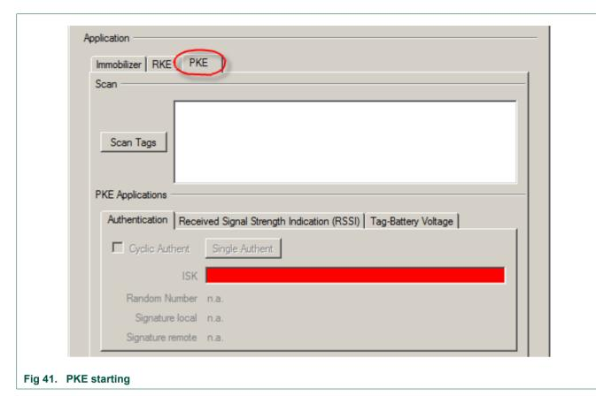
The window contains two sections: The upper section shows the currently configured infrastructure to run the PKE applet. The LF-Immo-Link base station is needed as uplink channel. The UHF RKE/PKE-Link base station is needed as downlink channel. The Tag window allows choosing the Transponder family.
