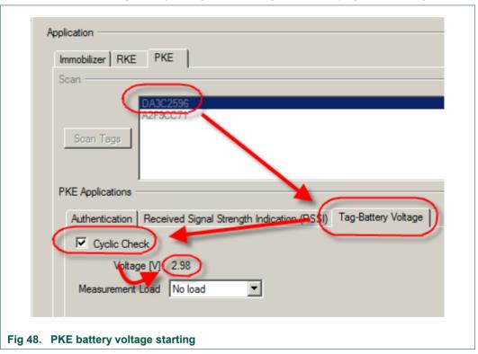
Select different loads for the Tag battery voltage measurement using the Measurement Load combo box. This setting can be changed during a running measurement (Fig 49a).
