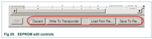
To enter a new value, just scroll to the page of interest and double-click inside the cell in the column Content and enter the new value. Modify any other page if required. To actually write the changes to the transponder, select Write To Transponder. To discard the changes made, click Discard.
