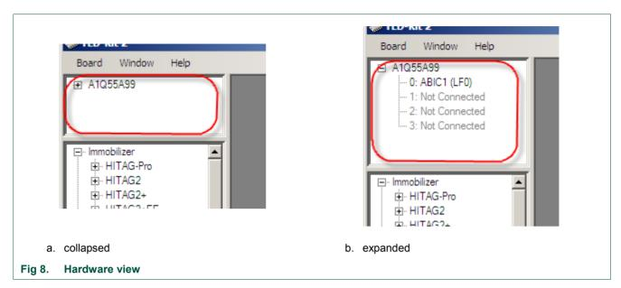
Note: TED-Kit 2 boxes can be plugged-in before or after starting the GUI. They are automatically detected. The hardware can also be removed at any time while the GUI is running.
