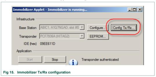
A new window opens and gives access to all communication settings of the LF-Link available. The settings are separated in Transmission to Transponder (Tx) and Reception from Transponder (Rx), see Fig 16.
