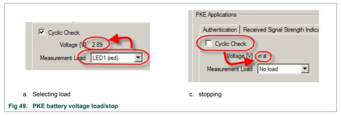
Disabling the Cyclic Check checkbox stops the Tag battery voltage measurement. The current voltage is no longer available (Fig 49b).
