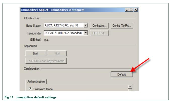
This sets the default values (for the selected transponder) for the authentication, transmission and reception parameters at once.
