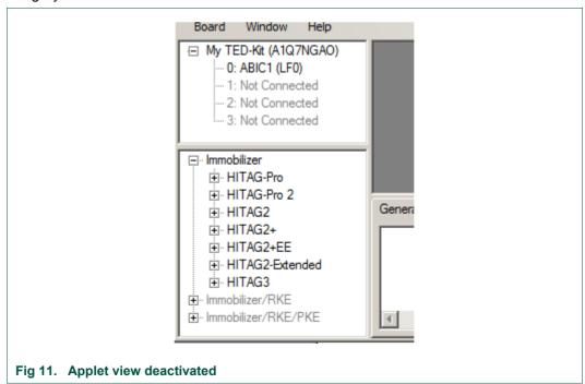
In Fig 11 there is one TED-Kit 2 box connected with one ABIC1 base station XBoard. Thus, the Immobilizer applet could be started.
