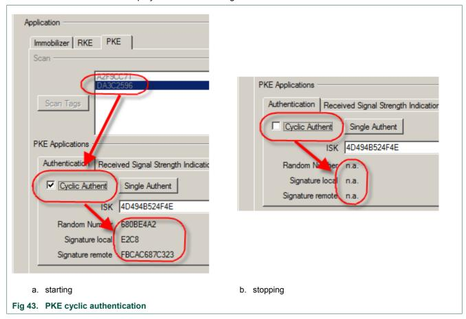
Disabling the Cyclic Authent checkbox stops the cyclic authentication. Exchanged values are no longer available (Fig 43b).
