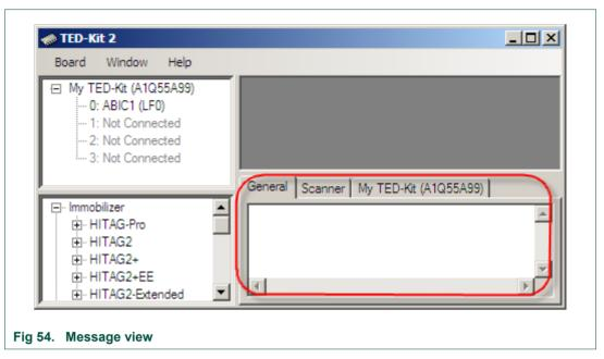
Several tabs are used to organize the messages and make reading them simpler. Two tabs always exist: The leftmost tab named General shows status messages from the GUI software itself.
