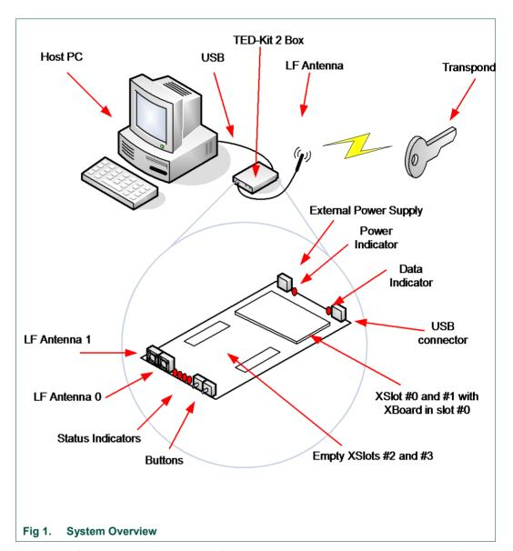
The host PC running the TED-Kit 2 software connects with the TED-Kit 2 box via USB. One or two external LF antennas are connected (depending on the internal configuration). Via the antenna, the TED-Kit 2 box exchanges data with the transponder IC found in e.g. a key.
