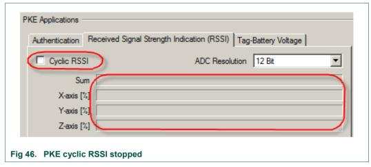
Select different ADC resolutions for the RSSI measurements using the ADC Resolution combo box. This setting is only enabled when the RSSI measurement is disabled (Fig 47).
