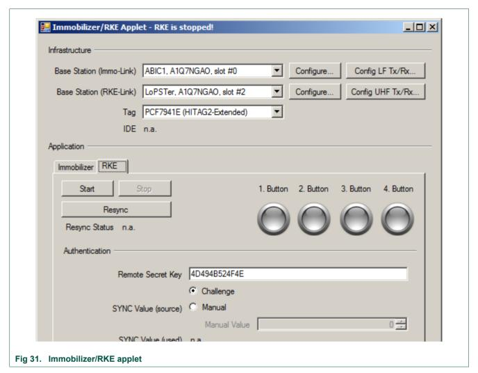
The window contains two sections: The upper section shows the currently configured infrastructure to run the RKE applet. The LF-Immo-Link base station is needed for the Tag-resynchronization. The UHF RKE/PKE-Link base station is need for the one-way RKE application itself. The Tag combo box allows choosing the transponder family.
