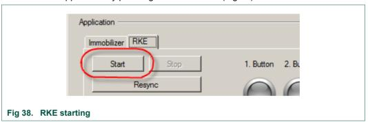
After the application was started any button on the tag can be pressed and the corresponding LED display will light up in the GUI like shown below. Additional the polling status will be displayed and should be OK.
