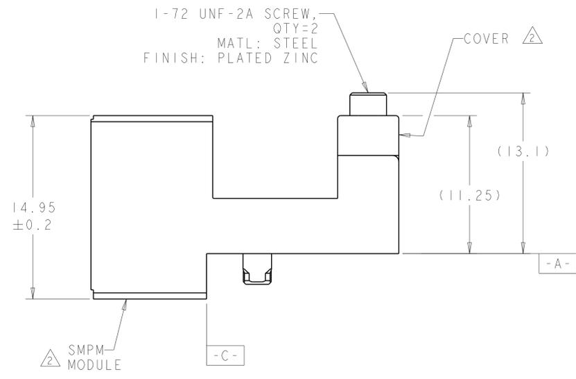
1 THE 2.25 FEATURE, [-A-], IS A TYPICAL HSR FAMILY LOCATING FEATURE. IN OTHER APPLICATIONS OF THIS MODULE A DIFFERENT FEATURE MAY BE USED FOR ESTABLISHING CORRECT LOCATION. THE [14.75] DIMENSION MAY BE REPLACED WITH OTHER VALUES FOR LOCATING THIS MODULE IN DIFFERENT POCKETS OF VARIOUS HSR CONFIGURATIONS.
