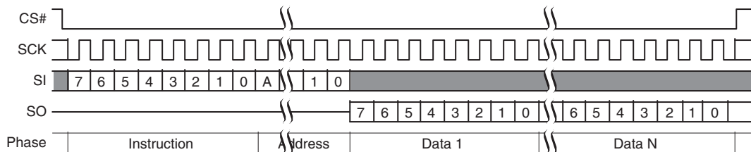
Figure 67. Read Command Sequence (READ 03h or 13h)
