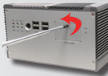
Unscrew and pull down the door
