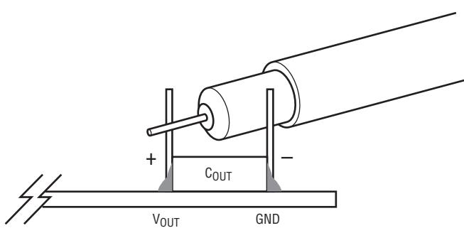
Figure 3. Measuring Input or Output Ripple Across Terminals or Directly Across Ceramic Capacitor
