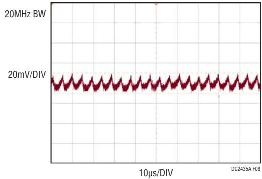
**Figure 8. DC2435A-A  $V_{OUT1}$  Voltage Ripple at  $V_{IN} = 14V$**
