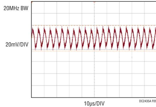
**Figure 9. DC2435A-A  $V_{OUT1}$  Voltage Ripple at  $V_{IN} = 48V$**
