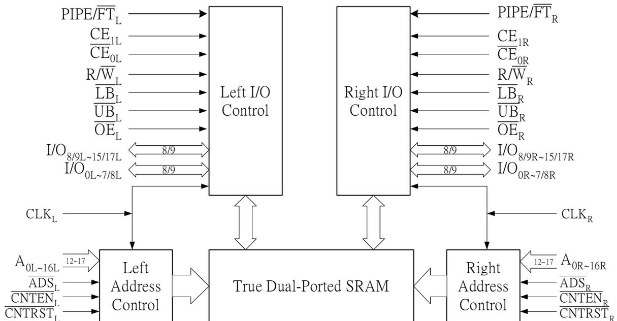
Note 1: LB<sub>R</sub> and UB<sub>R</sub> are for 16/18 bit devices only.
