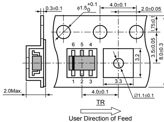
**TAPING REEL DIMENSIONS REUSE REEL (EIAJ-RRM-08Bc)**
