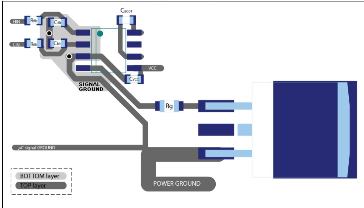
Figure 8. Suggested PCB layout (SO-14)
