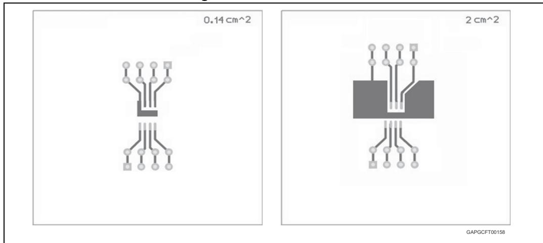
1. Layout condition of  $R_{th}$  and  $Z_{th}$  measurements (PCB: double layer, thermal vias, FR4 area = 48 mm x 48 mm, PCB thickness = 2 mm, Cu thickness = 35  $\mu\text{m}$  (front and back side), Cu thickness on vias 25  $\mu\text{m}$ , Footprint dimension 4.1 mm x 6.5 mm).
