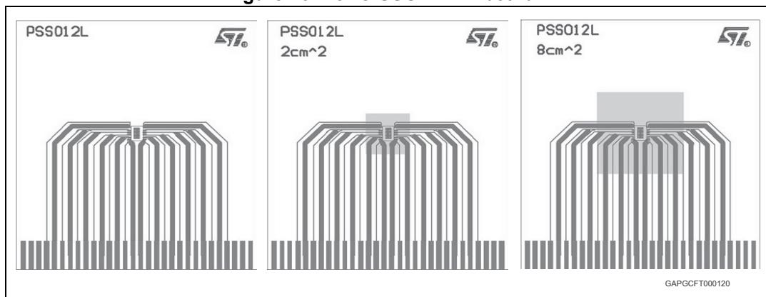
1. Layout condition of  $R_{th}$  and  $Z_{th}$  measurements (PCB: double layer, thermal vias, FR4 area = 77 mm x 86 mm, PCB thickness = 1.6 mm, Cu thickness = 70  $\mu$ m (front and back side), thermal vias separation 1.2 mm, thermal via diameter 0.3 mm +/- 0.08 mm, Cu thickness on vias 25  $\mu$ m, footprint dimension 4.1 mm x 6.5 mm).
