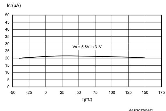
**Figure 19.  $I_{dr}$  vs.  $T_j$**
