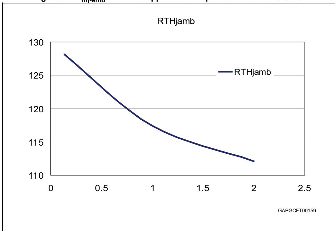
**Figure 32. SO-8 thermal impedance junction ambient single pulse**
