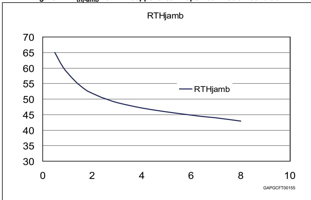
**Figure 28. PowerSSO-12 thermal impedance junction ambient single pulse**
