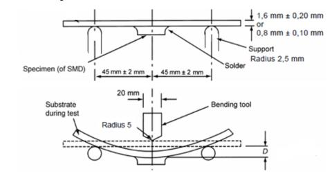
This substrate bending test is for all size of WCAP-CSST.
