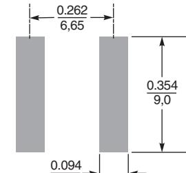
Dimensions are in  $\frac{\text{inches}}{\text{mm}}$
