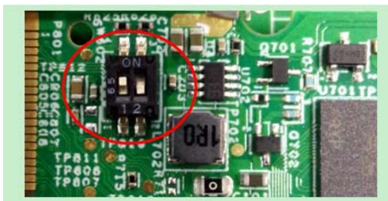
Figure 4. SW602 boot mode settings
