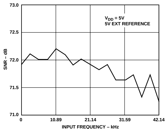
Figure 3. SNR vs. Input Frequency
