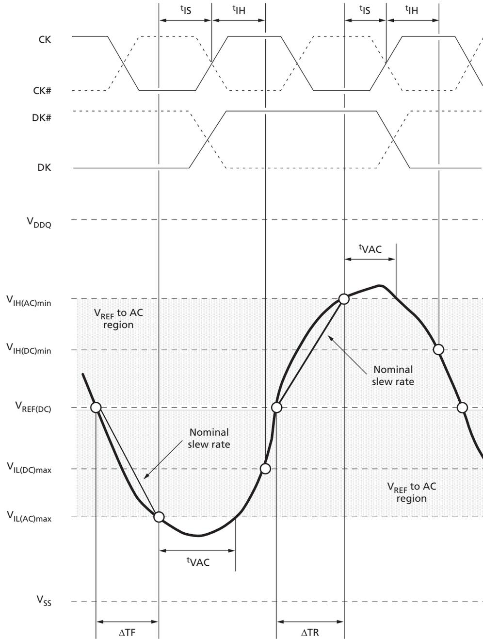
$$\text{Setup slew rate falling signal} = \frac{V_{REF(DC)} - V_{IL(AC)max}}{\Delta TF}$$
