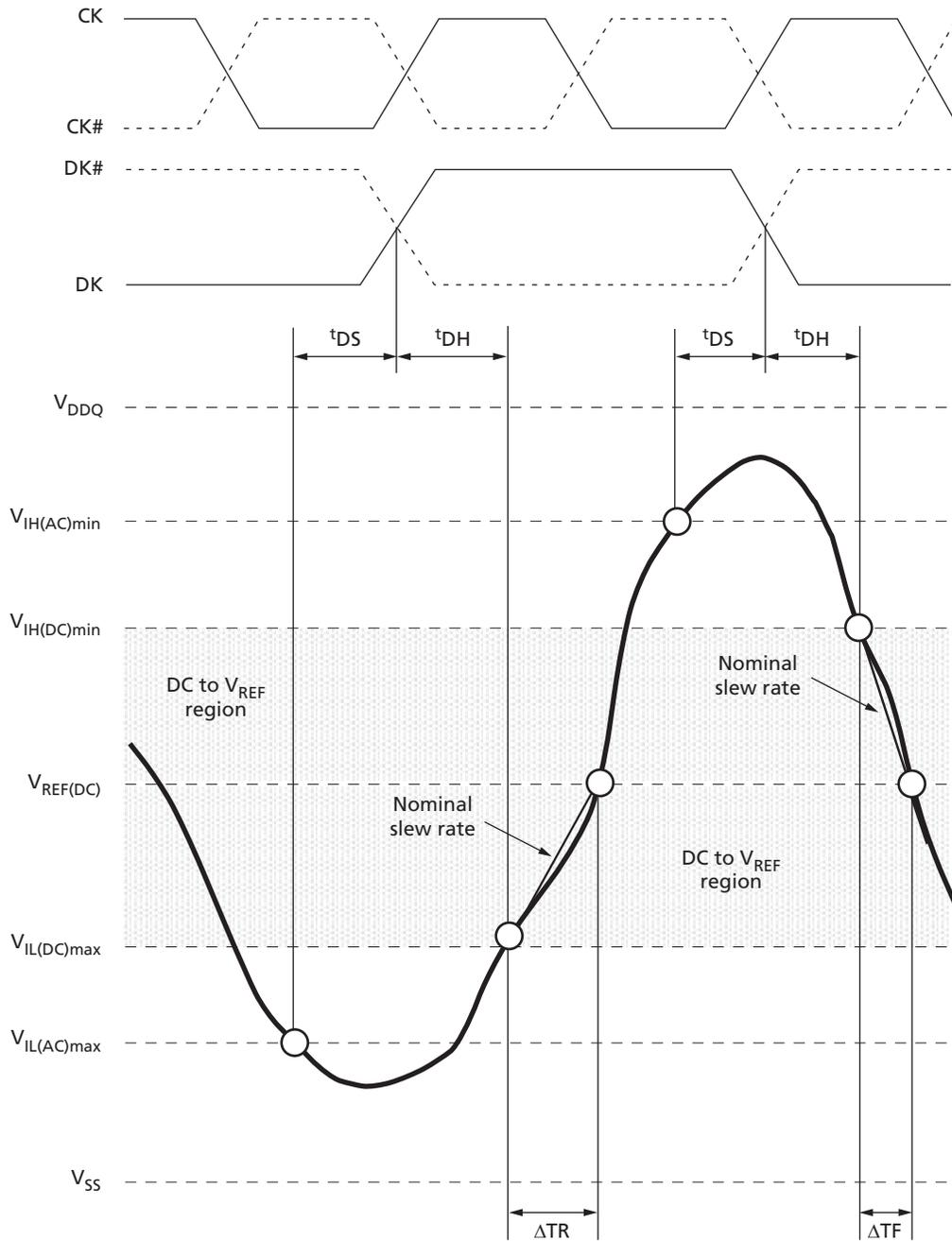
$$\text{Hold slew rate rising signal} = \frac{V_{REF(DC)} - V_{IL(DC)max}}{\Delta TR}$$
