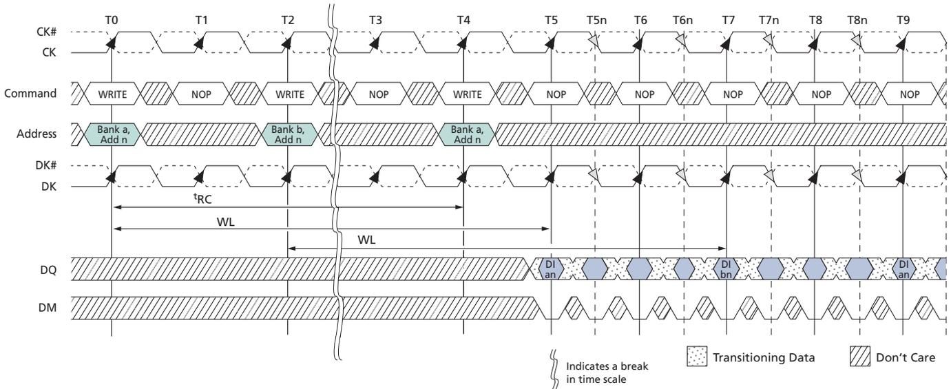
Note: 1. DI an (or bn or cn) = data-in for bank a (or b or c) and address n.
