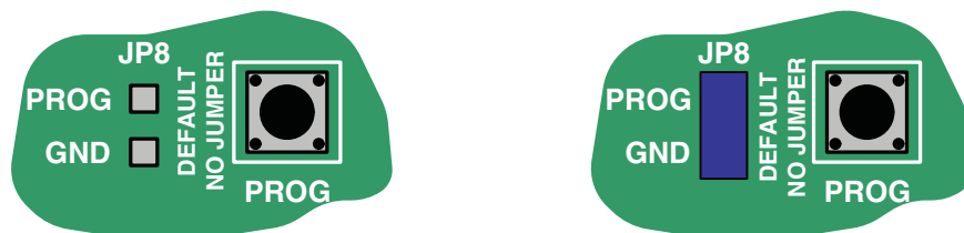
a) No Jumper: FPGA Operational (default)
