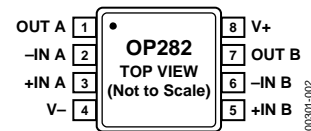
Figure 2. 8-Lead MSOP [RM-8]
