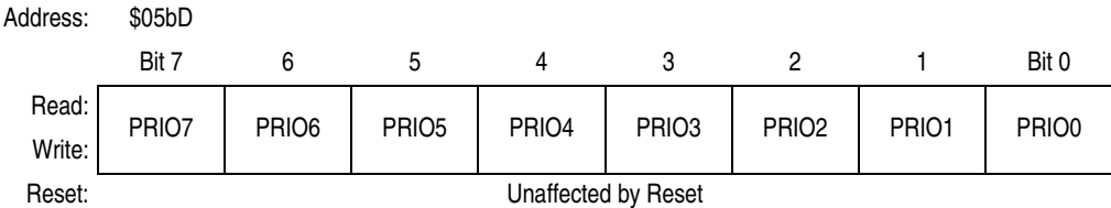
Figure 23-13. Transmit Buffer Priority Register (TBPR)
