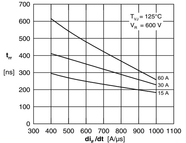
Fig. 10 Typ. recovery time  $t_{rr}$  versus  $di/dt$
