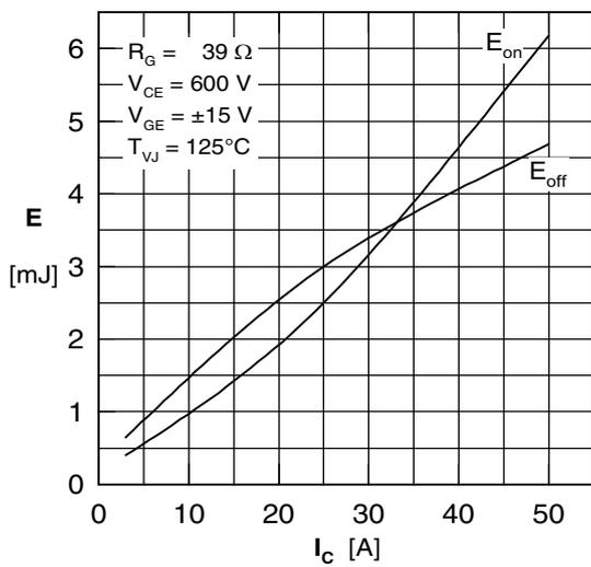
Fig. 5 Typ. switching energy vs. collector current
