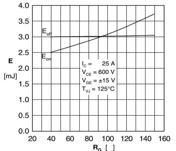
Fig. 6 Typ. switching energy vs. gate resistance
