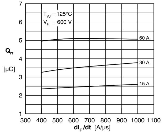
Fig. 8 Typ. reverse recov.charge  $Q_{rr}$  vs.  $di/dt$
