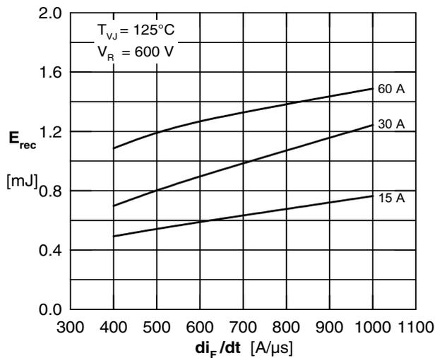
Fig. 11 Typ. recovery energy  $E_{rec}$  versus  $di/dt$
