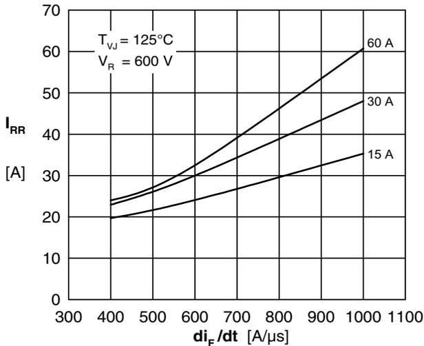
Fig. 9 Typ. peak reverse current  $I_{RRM}$  vs.  $di/dt$
