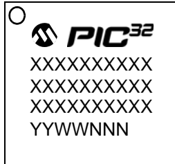
64-Lead QFN (9x9x0.9 mm)
