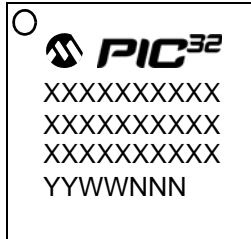
64-Lead QFN (9x9x0.9 mm)
