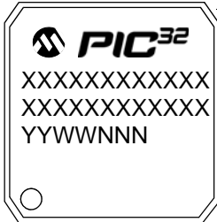
100-Lead TQFP (12x12x1 mm)
