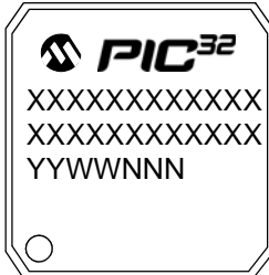
100-Lead TQFP (12x12x1 mm)
