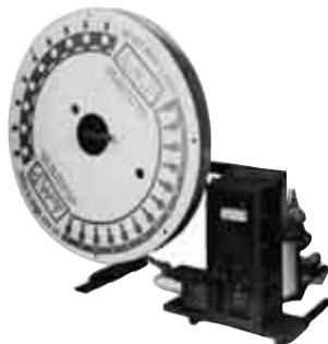
The semiautomatic power applicator is designed to produce a carefully controlled uniform pressure crimp while providing a high rate of production. The applicator features matching dies that fully bottom at the completion of the crimp to provide proper crimp height. The one die set is fully adjustable to provide the full range of crimp heights for all wire sizes.
